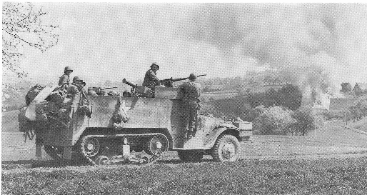
A light machine gun squad of the 61st Armored Inf. Bn. move forward through the German countryside on 17 April 1945. The half-track would appear to be an older M3 (winch) which has been rebuilt with an M49 ring mount and pulpit. Newly manufactured M3A1s had mine racks fitted to the hull side, which this vehicle, like many M3s, lacks. The half-track's armament includes both an air-cooled and a water-cooled .30cal. Browning. (US Signal Corps)
