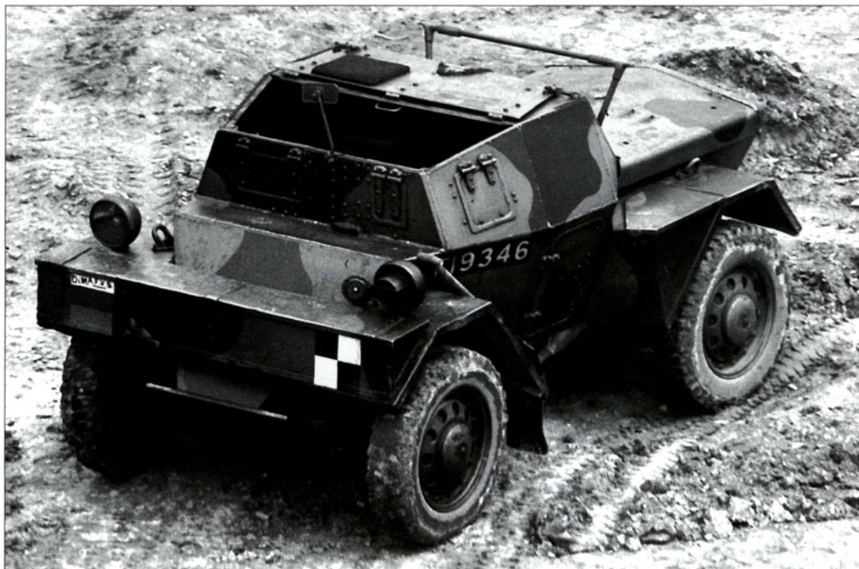
Also from the Daimler stable was the Dingo scout car, used in large numbers by 52 (Lowland) Recce and, to a much lesser extent, by other units. Capable of 55mph, it had a range of 200 miles and a two-man crew. This vehicle does not yet carry unit markings. (IWM STT 8201)
